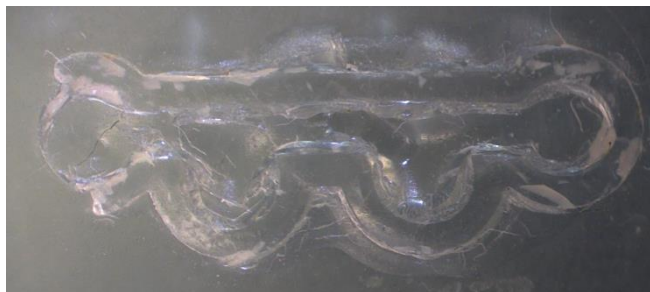
Figure 6-5. Patterning channel and chamber on a PMMA substrate using UE technique.
