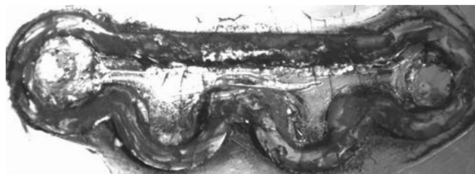
Figure 6-6. Patterning channel and chamber on a coated PMMA substrate with graphite using UE technique.
